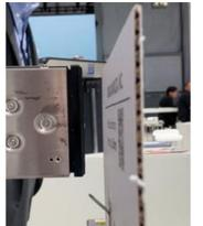
Our thin-film printheads achieve clear print even with high gaps, ensuring application to the cardboard conveyance process
