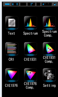
Measuring Mode Selection Screen
