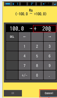
Selected CRI Value Input Screen (outside the setting range)
