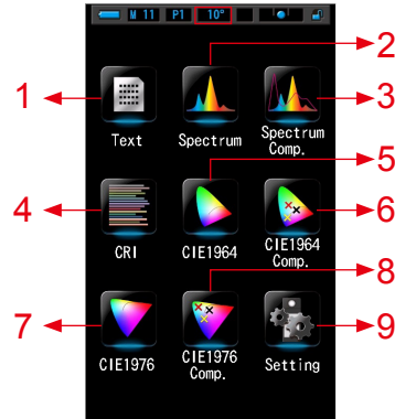
Display Mode Selection Screen (10°)
