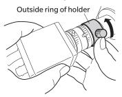
While the tightening screw of the holder is still loose, rotate the camera while monitoring the shooting screen to align the rotation direction of the camera.
