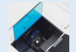
Transmittance Measurement: The CM-3600A/CM-3610A employs the d:0° geometry (diffuse illumination, 0° viewing), which conforms to CIE, ASTM, DIN and JIS standards.
